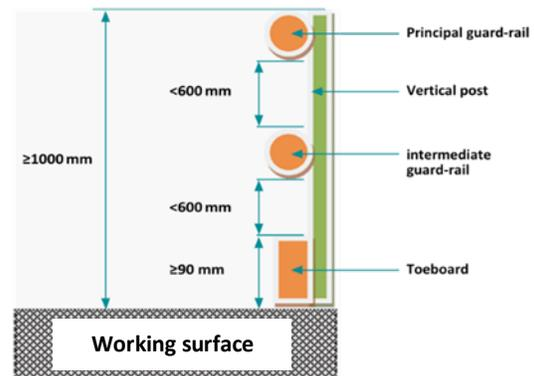
Figure 4 Dimension requirements for a temporary edge protection
