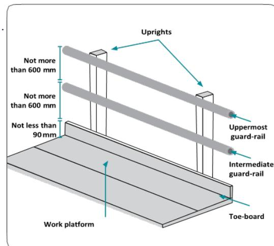
Figure 8 Dimensions of working platform
