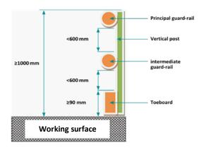
Figure 4 Dimension requirements for a temporary edge protection
