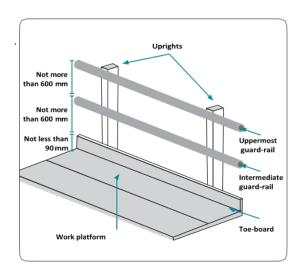
Figure 8 Dimensions of working platform
