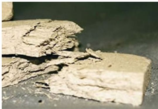
Pieces of Asbestos Insulation Board (AIB)
