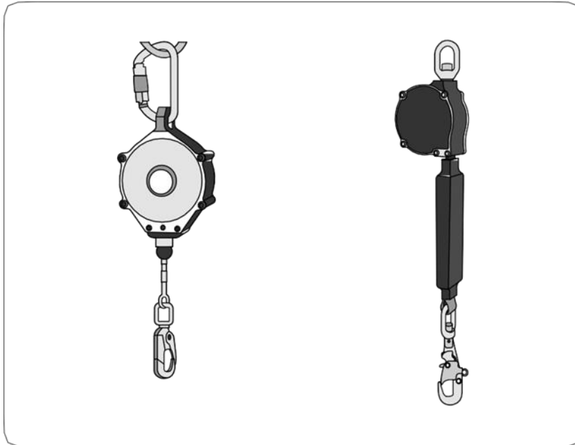
Figure 6.3: Examples of self-retracting lifelines.
