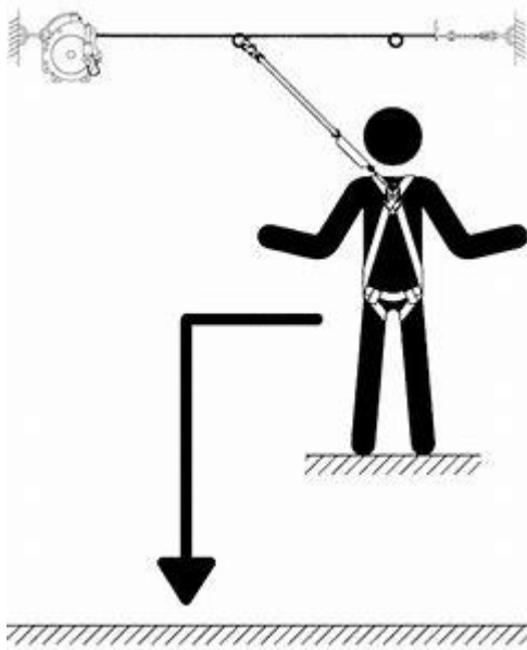
Figure 6.2: An example of a horizontal lifeline.
