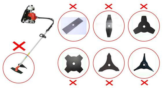
Figure 1 – Type of metal blades<sup>4</sup> not recommended (the "knife blades")
