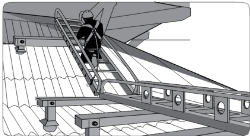
Figure 11.2: Crawler boards, gangways and perimeter guard-rails can enhance safety for work on pitched roofs.
