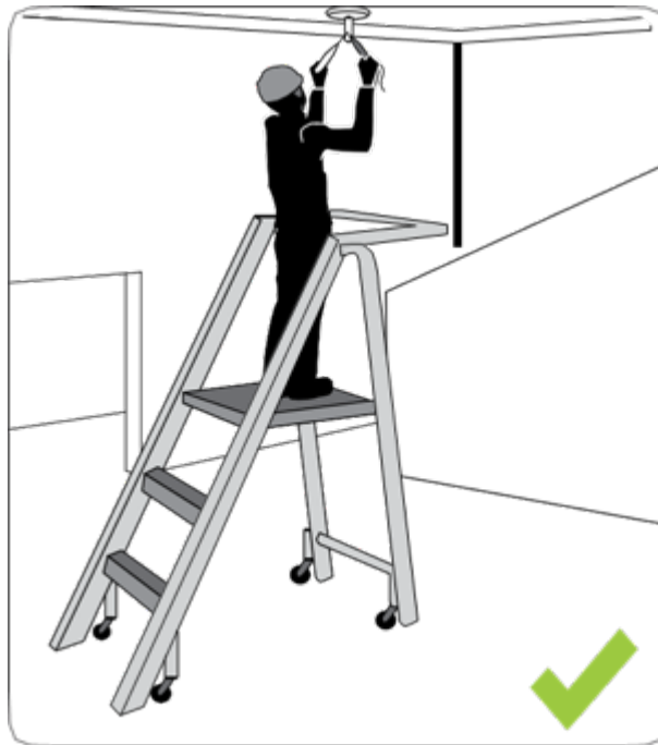
Figure 10.2: A step platform can provide a more stable work surface.
