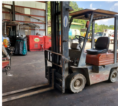
Photo 1 of forklift Truck with worn-out tyres
